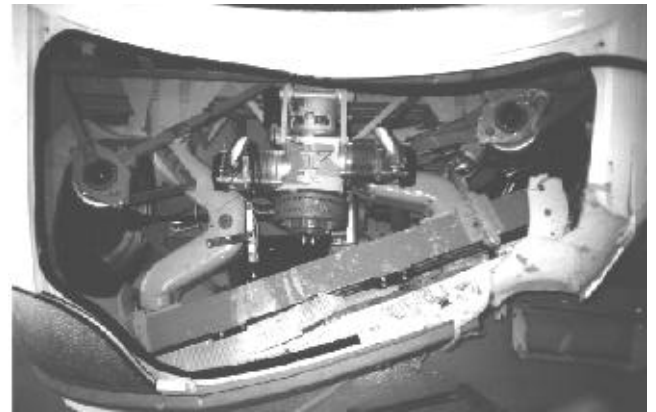
Figure 12: CRATCH - deformation of the front beams.
